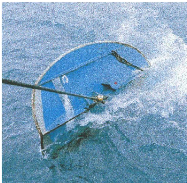
Figura 4. Puerta de arrastre Poly Ice Concord (Hampidjan).
