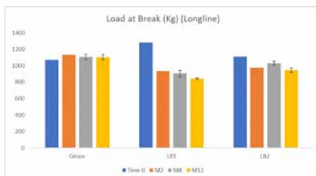
Figure 1. Monitoring tensile of ropes in the sea culture for 1 year in longline. Load at break (kg) vs. months (M).
