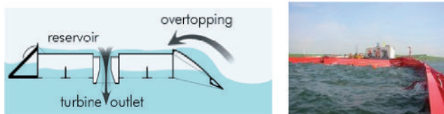
Figure 16 Wave Dragon System. From http://www.wavedragon.net/ .
