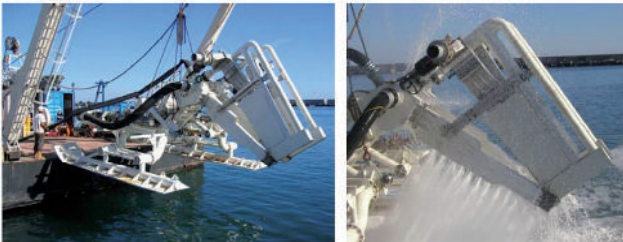
Figure 11. Towed Jetting Vehicle 06 by LD TravOcean (www.ldravocean.com).
