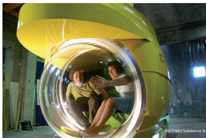
Figure 1. Image of unfinished submersible assembly and detail of visibility in the front acrylic window, in summer 2011
