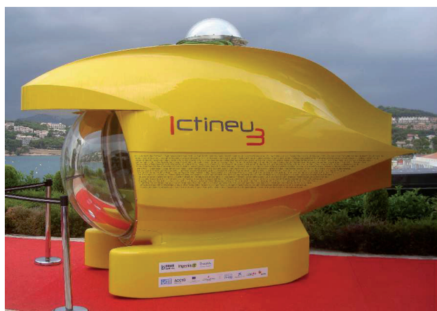
Figure 1. Image of unfinished submersible assembly and detail of visibility in the front acrylic window, in summer 2011
