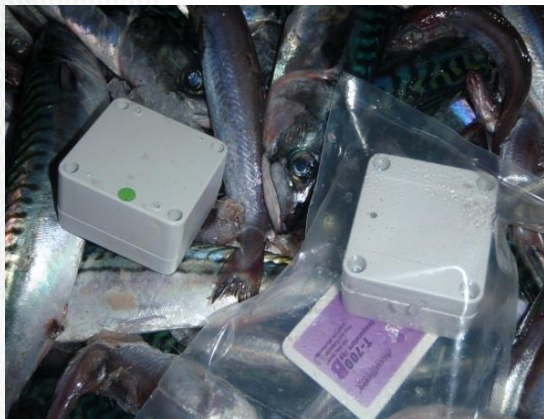
Data-loggers to measure T^a of the fish along the value chain
