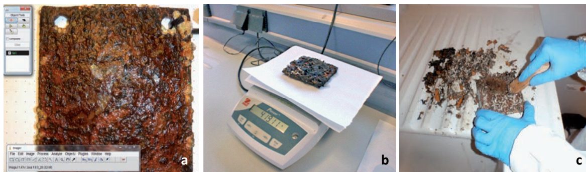
Fig. 5. Macrofouling evaluation. (a) Macrofouling cover estimation using the Java image processing software Image J, (b) weighing a panel covered with biofouling and (c) biofouling scraping for biomass calculation.
