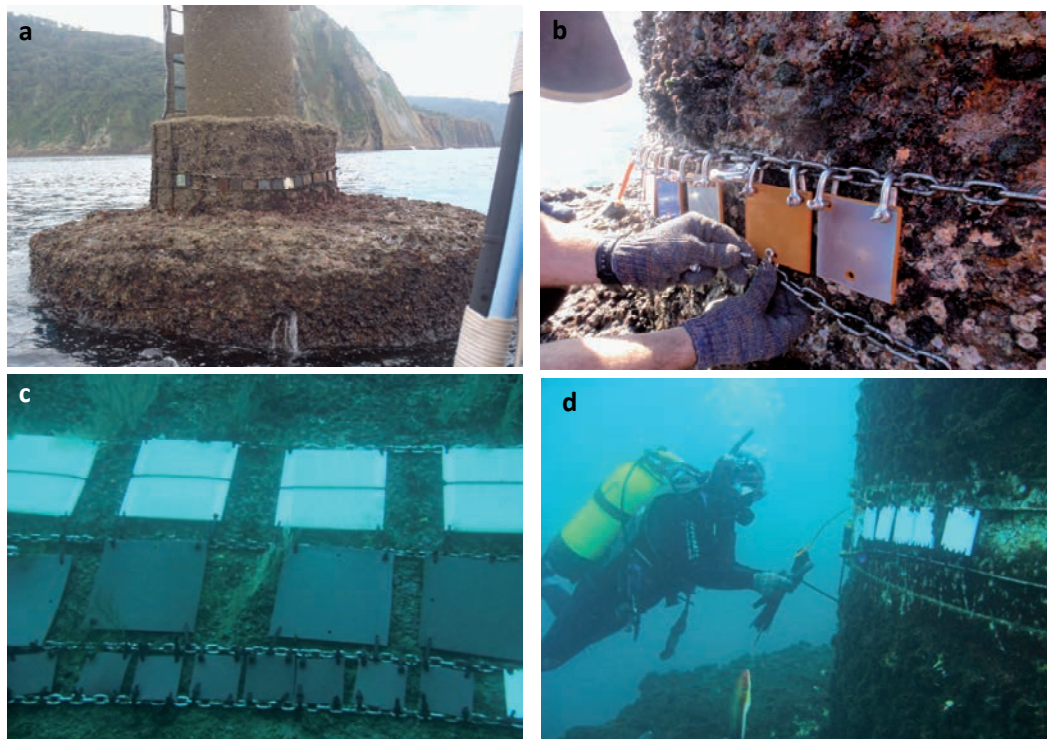
Fig. 3. Structures for the installation of different panels for biofouling formation studies at the OMS of Pasaia. (a) a structure consisting of two chains in which the panels are installed at the splash zone; (b) installation of the panels with shackles to the chains at the splash zone; (c) a structure composed of four chains showing panels of different size and material at a depth of 4 m; and (d) a diver attaching panels with plastic flanges to a cable at 20 m depth (OMS: Ocean-meteorological station).
